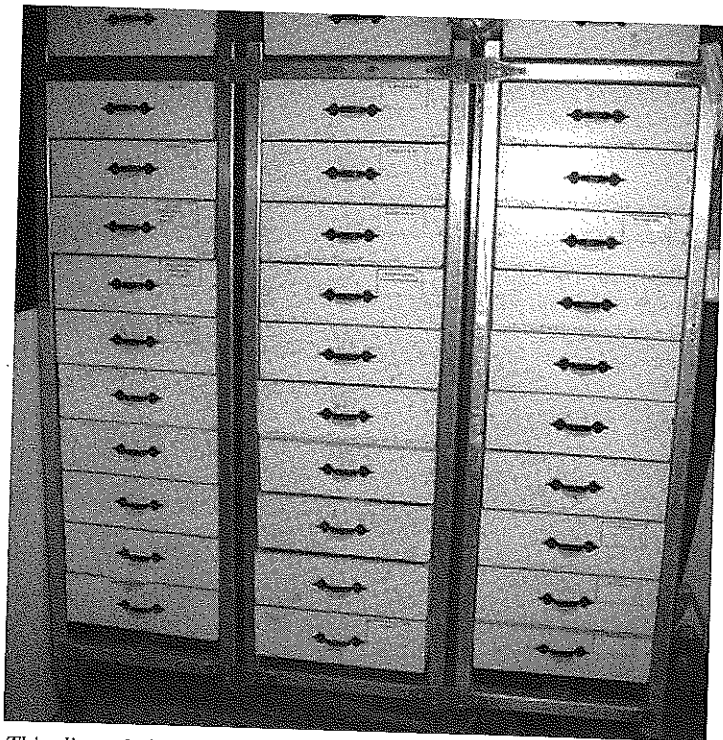
This discarded aluminum baker's cooling rack works well as a multi-drawer storage unit. Thin 1/4-inch plywood was used to make the 30 drawers. Three large bins on top are for large parts.
